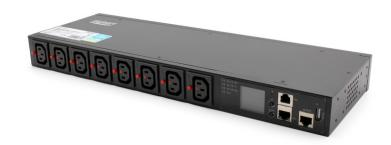
Power strip IPDU H enables switching on/off of outlets and power measurement via TCP/IP. The front panel is equipped with 8 IEC320 C13 outlets. Power ports are individually switchable through a network interface, SNMP, or directly using the button on the control panel. Integration with an additional device (DN-S-BOX) allows the connection of dedicated sensors to monitor: ambient temperature/humidity, door opening/closing, and detect the presence of water or smoke.
