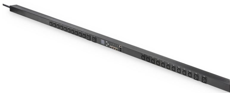
**Inlet monitored PDU, vertical, 16A, 20xC13, 4xC19 3m cable, IEC60309 16A plug**
