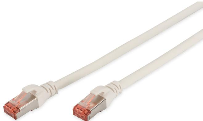
**CAT 6 S-FTP patch cord, Cu, LSZH AWG 27/7, length 7 m, color white**
