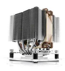
L.N.A. (+/- 10%): 1550 RPM Min. Rotational Speed (PWM, +/-20%): 400 RPM Max. Airflow: 78,9 m³/h Max. Airflow with L.N.A.: 62,6 m³/h Max. Acoustical Noise: 22,8 dB(A) Max. Acoustical Noise with L.N.A.: 16,3 dB(A) Input Power: 1,2 W Voltage Range: 12 V MTBF: > 150.000 h
