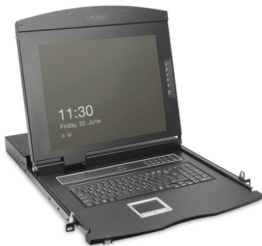
**Modularized 43,2cm (19") HD TFT console with 8 port CAT5,with TR keyboard, RAL 9005 black**
