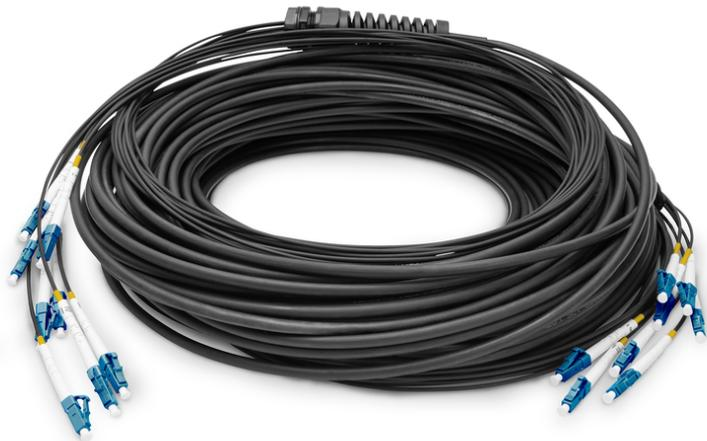
**Breakout Kabel 8 Fasern, SM G.657.A1 LC/UPC-LC/UPC, universal, Farbe: schwarz, 100m**
