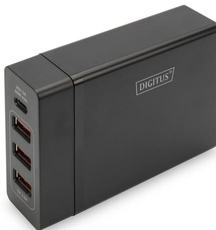
**4-Port USB Charger, 72W, 1xUSB-C (Power Delivery), 5,9,15,20V/3A and 3x USB-A 5V/2.4A, black**
