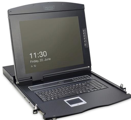
**modularized 43,2cm (17") TFT console without keyboard and KVM module, RAL 9005 black**
