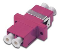
FO coupler, duplex, LC to LC, MM, violet, OM4 ceramic sleeve, polymer housing, incl. screws
