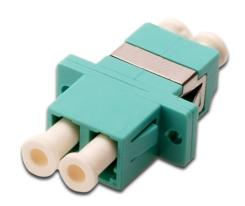
FO coupler, duplex, LC to LC, MM, color aqua, OM3 ceramic sleeve, polymer housing, incl. screws
