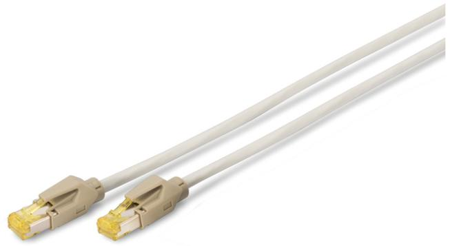
CAT 6A S-FTP Patchkabel DRAKA UC 900 SS FRNC, TM31 Cu, LSZH, AWG 27/7, Länge 7 m, Grau
