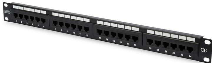
**CAT 6 Patch Panel, unshielded, 24-port RJ45, 8P8C, LSA, 1U, rack mount, bl, 482x44x109**
